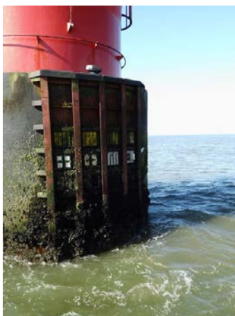
Figure 2: Test specimens in the coastal shipping region at the Alte Weser Lighthouse. © Fraunhofer IFAM
