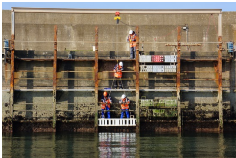
Figure 1: Outdoor weathering test stand at Westmole, Helgoland. © Fraunhofer IFAM
